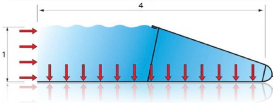
*The Water-Gate anti-flood dam deploys automatically once the water begins to flow.*
