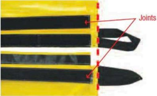
2. Both barriers must be aligned at the back. Make sure the joints are open.
